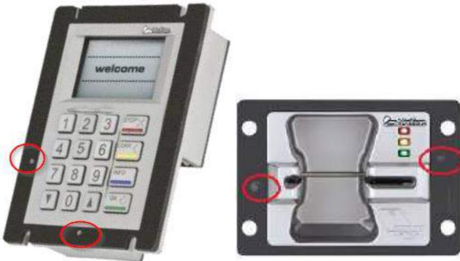
Make sure that the plates have been attached correctly and firmly. They must not be loose and must not come out during normal usage of the terminal.
